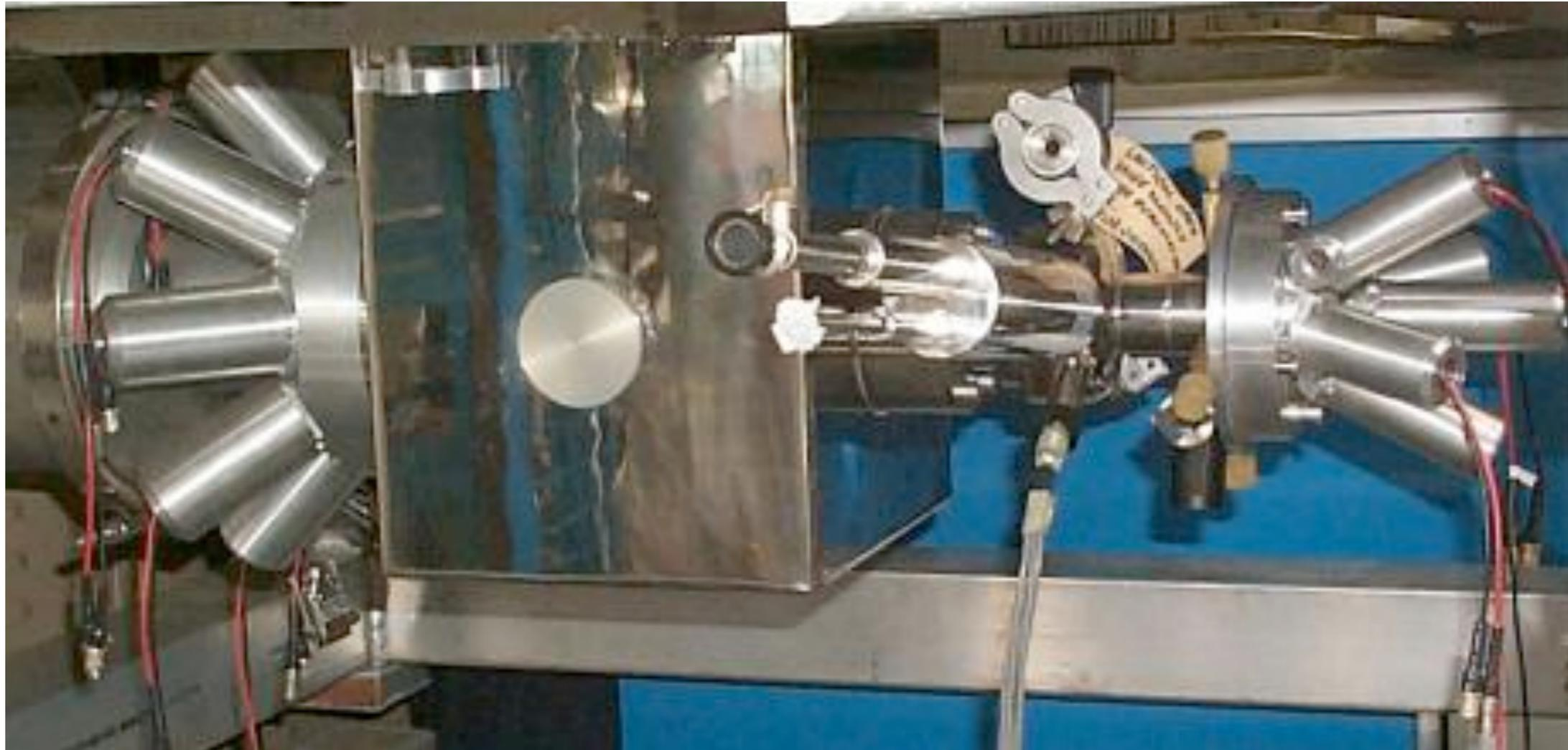
Fields of up to 8 T are now available, requiring a “business end” of the spectrometer only 3 cm in diameter (so that 30-50 MeV decay positron orbits don’t “curl up” and miss the detectors) and a time resolution of  $\sim 150$  ps. Muonium precession frequencies of over 2 GHz have been studied.
