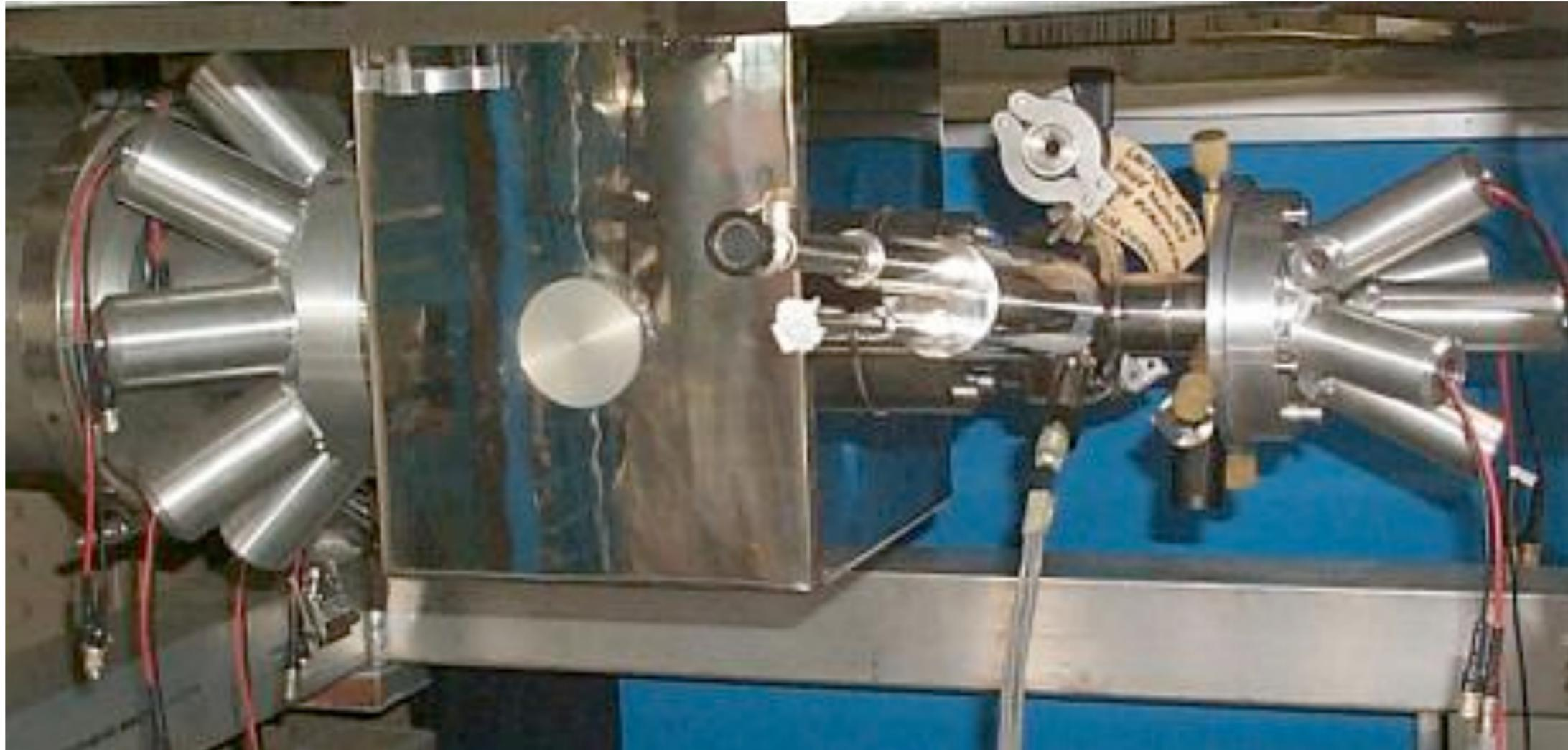
Fields of up to 10 T are now available, requiring a “business end” of the spectrometer  $< 3$  cm in diameter (so that 30-50 MeV decay positron orbits don’t “curl up” and miss the detectors) and a time resolution of  $\sim 150$  ps. Muonium precession frequencies of over 2 GHz have been studied.
