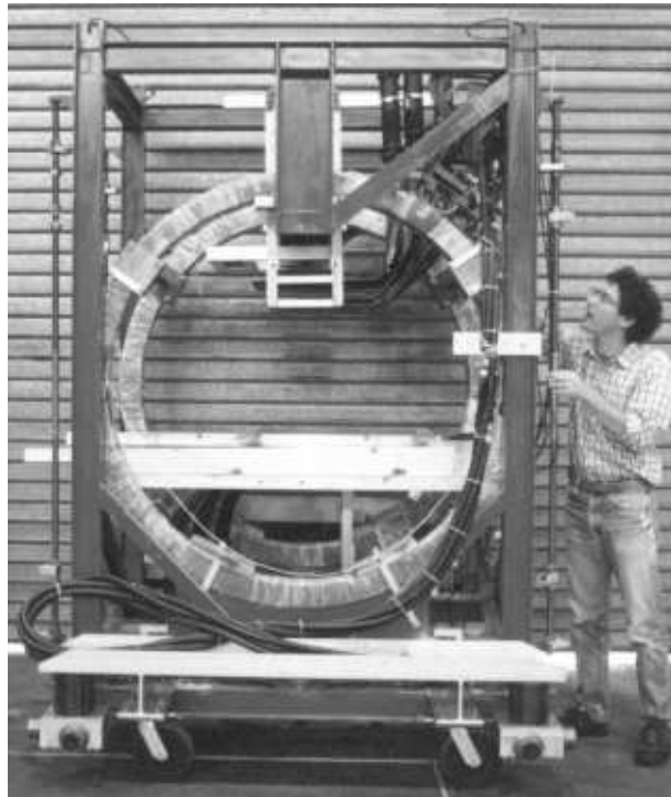
Figure 4.6: The Gas Cart, with the light correction coils dismantled.
