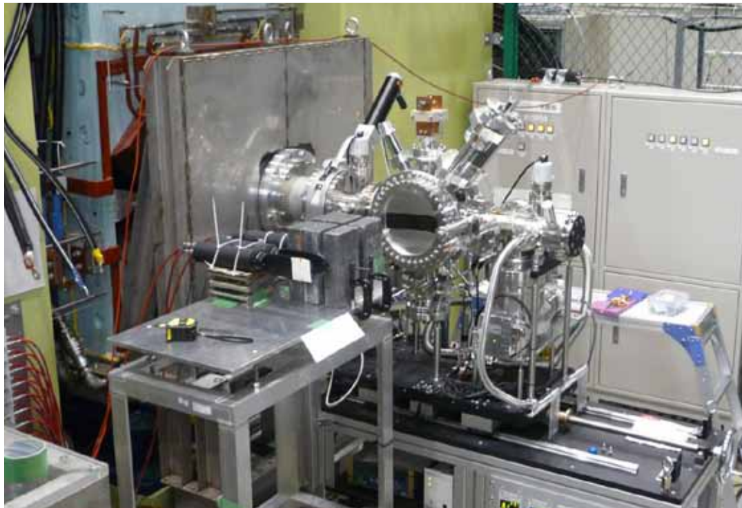
Vacuum chamber for investigating Mu production rate from W foil
